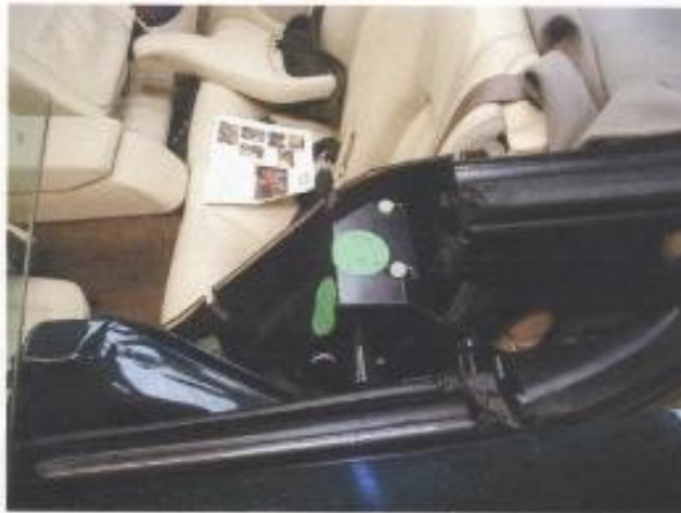
Fig:5 View of metal plate to be drilled shown here with green sticker attached (top one).
