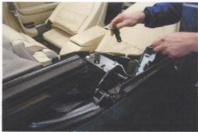
Fig:2 Showing leather top mounting removed (driver's side) and the already drilled holes. Engineer is holding larger piece of angle iron for fitting.
