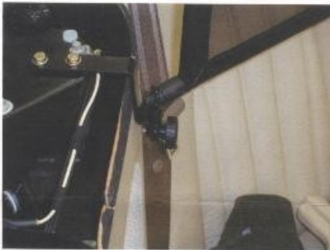
Fig:7 Fitting of large section of wind deflector through smaller piece of angle iron into larger piece of angle iron and held by thumb screw (driver side)
