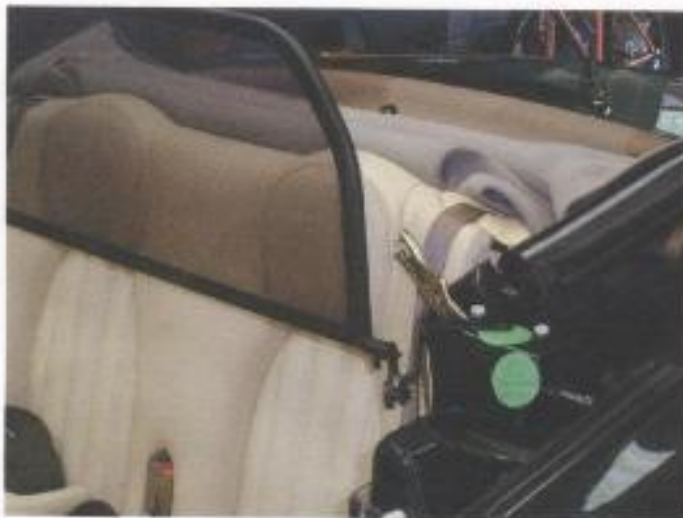
Fig:8 View showing test placement on passenger's side of wind deflector through pieces of angle iron prior to drilling. (held by clamp)
