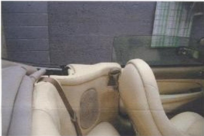
Fig:1 Showing leather top mounting to be removed complete with seat belt fitting
