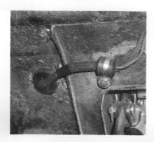
Remove the wires from the hydraulic brake light switch and pass them through the new hole. From inside the vehicle, place the rubber grommet over the two wires; and then install the grommet into the new hole. (We recommend the hole be sealed with black RTV or similar sealant.) Remove the
