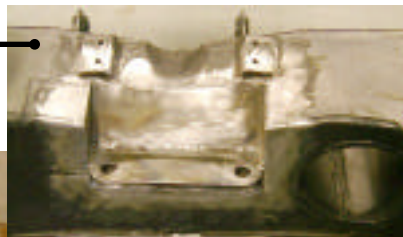
Gearbox rear mounting showing position from front of crossmember
